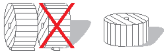
Do not lay drums flat on their sides, use proper stops to prevent drums rolling.
